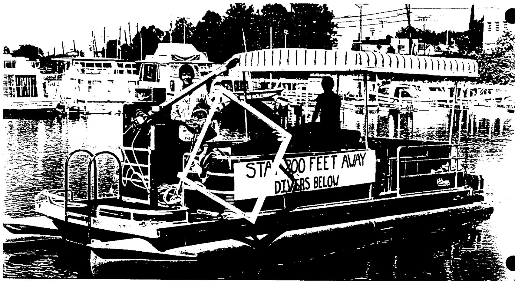
Figure 1. Illinois Natural History Survey River Diver, a 24-ft pontoon boat modified to support surface-supplied diving.
