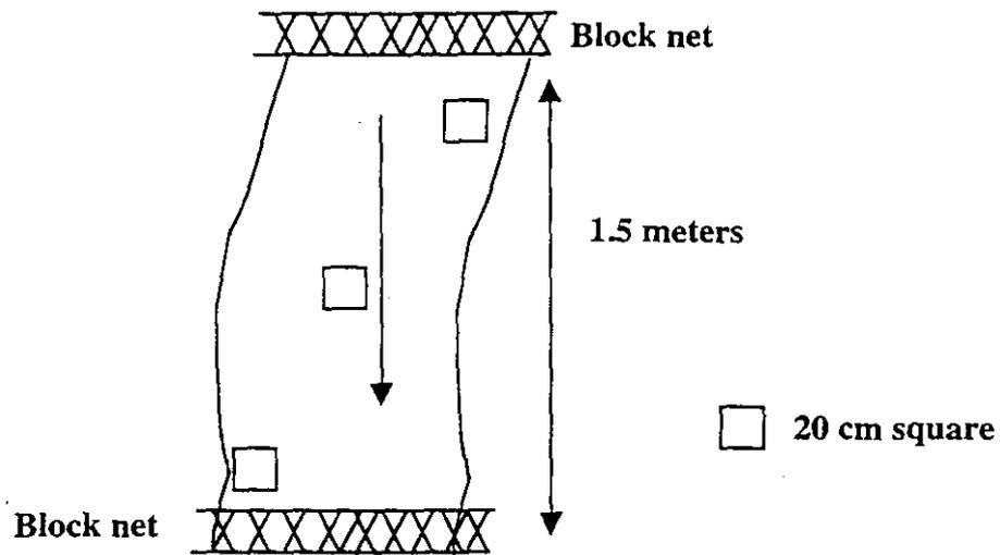
Figure 6. Diagram of the sampling procedure for each plot. Block nets were placed at both the upstream and downstream edge of the plot. A 20 cm square was positioned in the stream three times along a diagonal. At each square, cover and substrate were determined for the edges and center of the square to give a total of 15 measurements.
