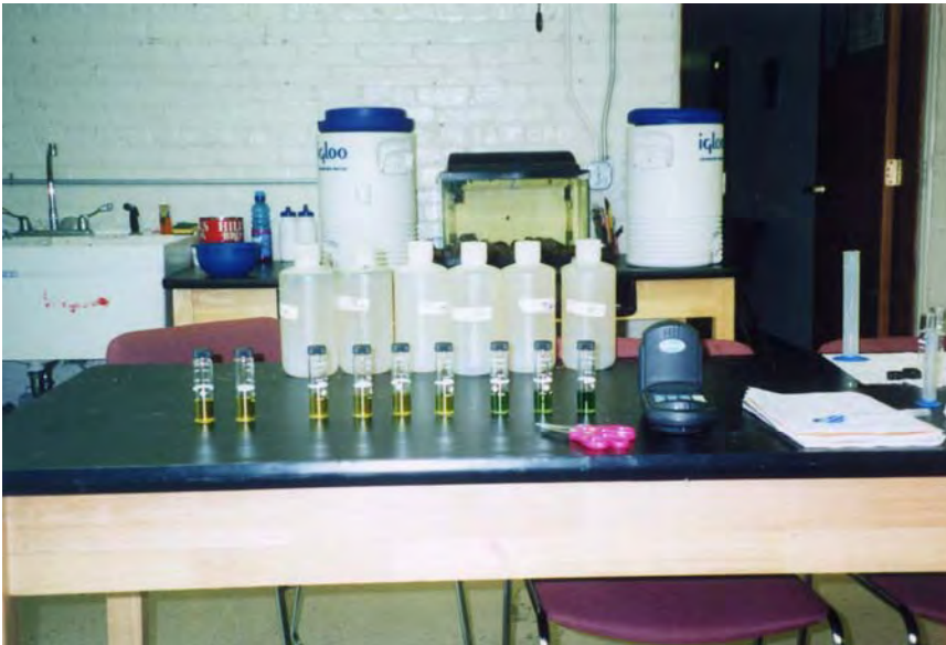
Fig. 4: Hach Test for Phosphate – An example of the set up for testing for phosphate using the Hach Method.
