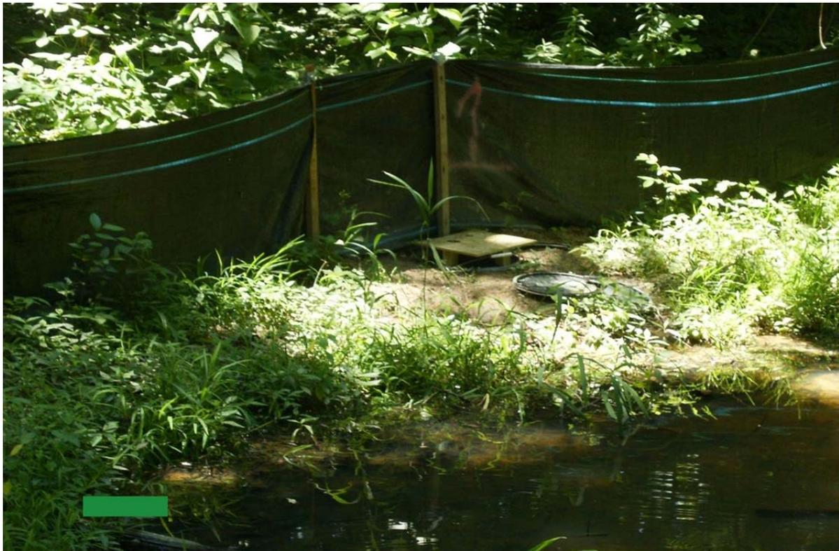
Figure 1: Drift fence constructed of black silt fencing and pitfall trap with modified bucket lid.
