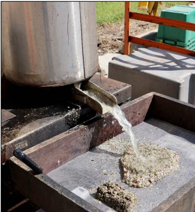
Various unique machines are used to clean different types of seeds. This one uses water to wash away to the fleshy seed coating and the seeds stay in the container
