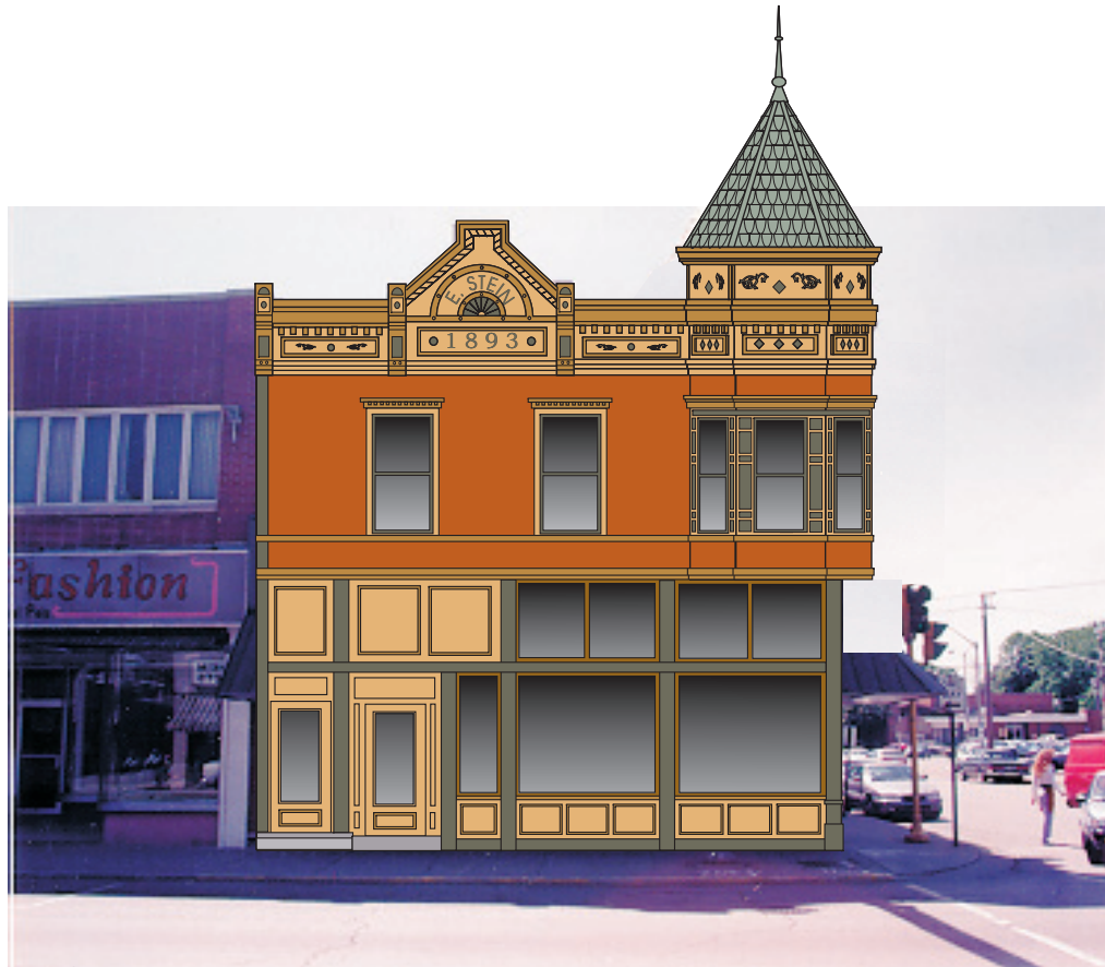
PROPOSED ELEVATIONS SHOWN WITH TRANSOM WINDOWS, WITHOUT AWNING
