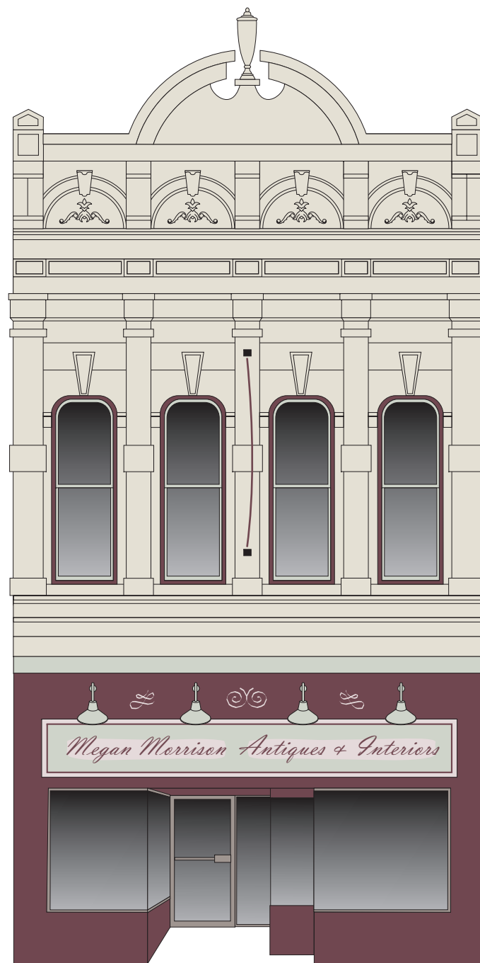
FLUSH-MOUNTED SIGN GOOSENECK FIXTURES
