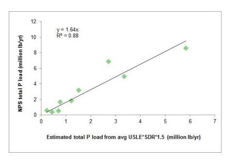
Figure 3.19. Annual average non-point source total phosphorus loads from the modified MLRAs plotted as a function of loads estimated from the average USLE erosion rates, cropland area, and SDR and assuming 1.5 lb total P/ton of sediment.
