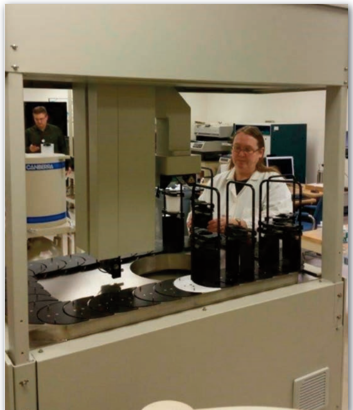
Kerrie Peacock, IEMA radiochemist, loads a sample on a gamma spectrometer.
