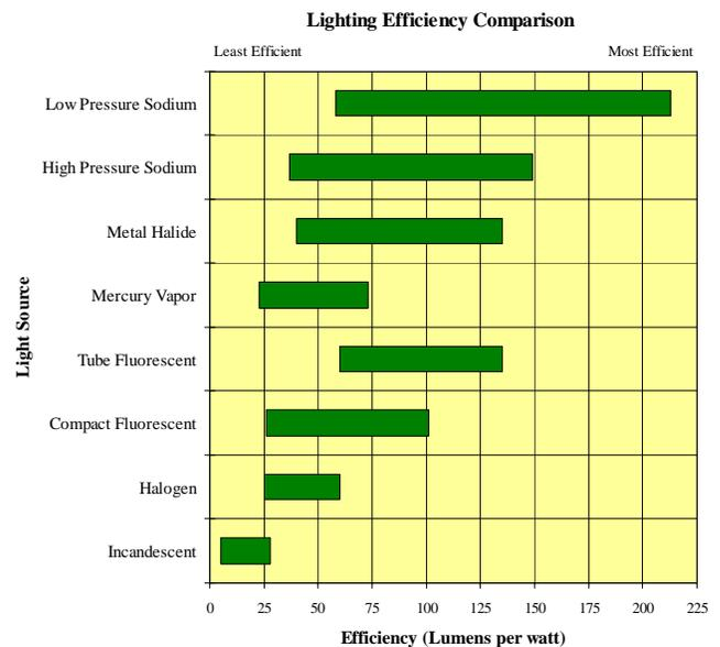
As the graph shows, incandescent are the least efficient lamps available. They provide an adequate range of lumens, but also, consume large amounts of watts in comparison to the amount of light they provide.
